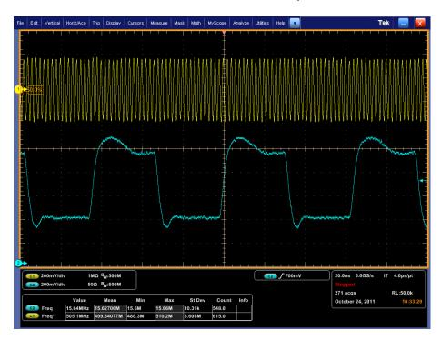
Channel 1 = 500 MHz clock Channel 2 =  $\div$ 32 output into 1M.
